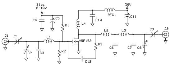
C1 C2 C8 - ARCO 463 C3 C7 - 25 pF ATC 100B C4 C10 C12 - 0.1uF 100Y SMT C5 - 1 uF 15WY tant C6 - 250 pF ATC 100B C9 - ARCO 462 C11 - 15uF 100Y Elect
