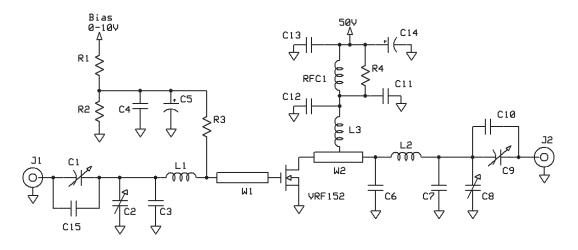
C1,2,8,9 - ARCO 463 20-180pF C3,7 - 120 pF ATC 100B C4,11-13 - 0.1uF 100Y SMT C5 - 1 uF 15WV tant C6, C15 - 47pF ATC 100B C10 - 150pF ATC 100B C14 - 15uF 100Y Elect W1 W2 - printed line 0.23"x 0.7" L1 - 4t #20 ga .25"d x .16"L ~120nH L2 - 5t #14 ga .312" dia x .45" ~135nH L3 -7 turns #16 ga 5/16" ID tight. ~250nH R1 R2 - 2.2k ohm 1/4W R3 - 22 ohm 1W SMT R4 - 2.2 ohm 2W RFC1 Fair-Rite 2961666631 (VK200-4B) PCB = FR-4 fiberglass-epoxy er = 4.6
